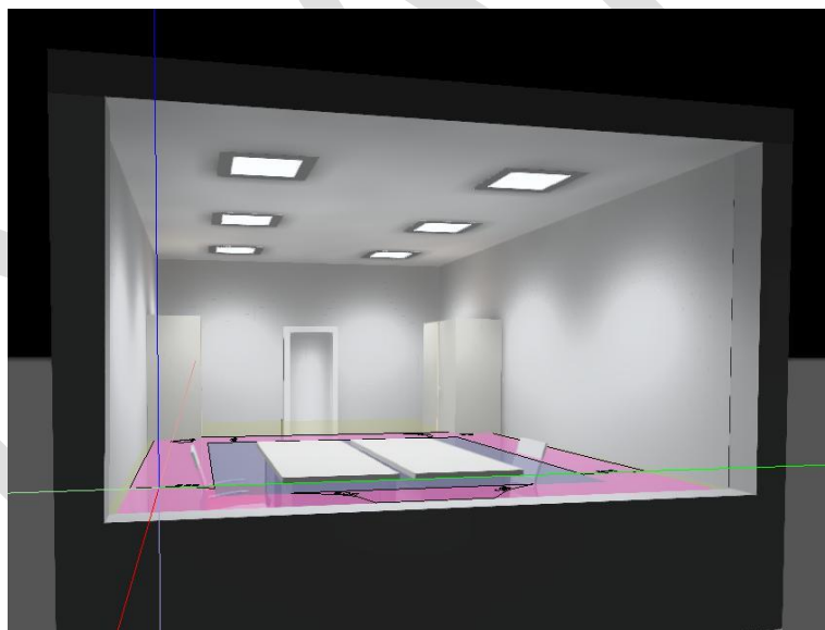
Figure 3-2: Cellular office with ceiling mounted luminaires reference design
