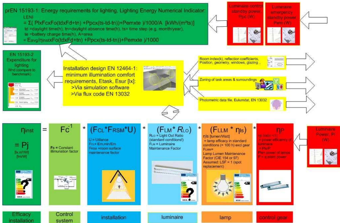
Figure 3-6 Formulas for modelling energy consumption in indoor lighting
